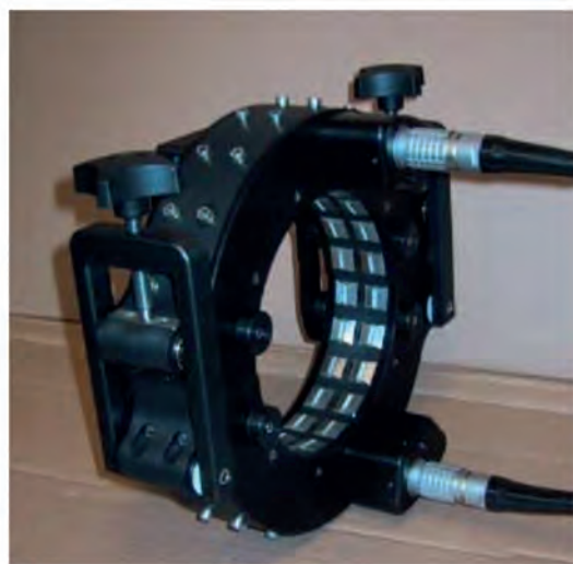
Theoretical analysis of ultrasonic wave modes in pipes and an early, rigidly clamped transducer system (courtesy of Cawley et al. Imperial College)
